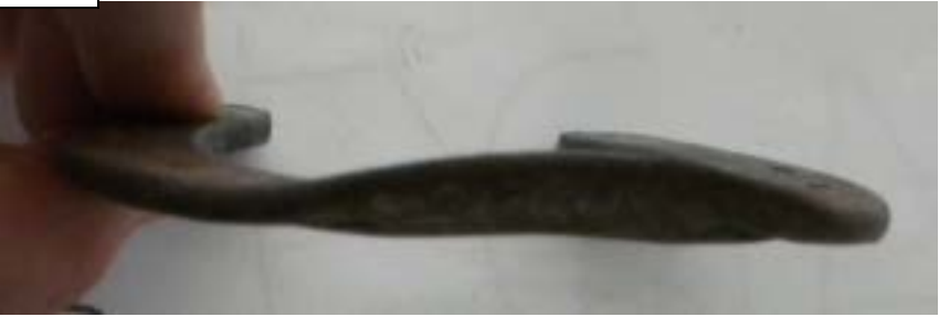
ILLEGAL Rocker Toe
